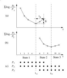
Figure 1: The scheme of the proposed decoding algorithm: (a) the end-point detection for state 1,  $t_5$ ; (b) the end-point detection for state 2,  $t_9$ ; and (c) the grid points for  $p_1$ ,  $p_2$  and  $p_3$  computations (dots).
